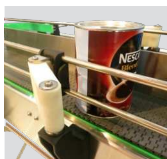
Conveyor guide rails
