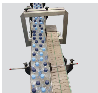
Slat chain conveyors
