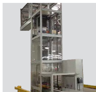
Continuous carton elevators
