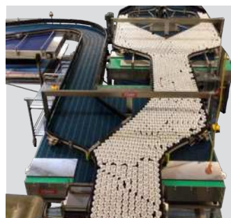
Mass flow conveyors
